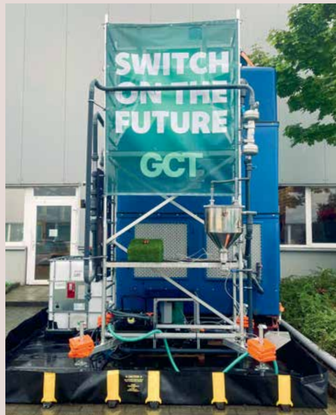
The DAC demonstration system in Essen boasts an annual capacity of 100 tonnes of carbon dioxide.
